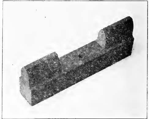
FIG. 560. JIG FOR SHAPING SPUR GEAR TEETH.
